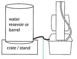
Attach 19mm poly hose from resevoir to ball float (supplied) on evaporative unit.
