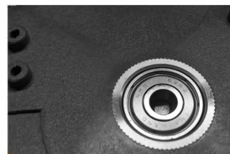
Heavy Duty NMB Ball Bearing
